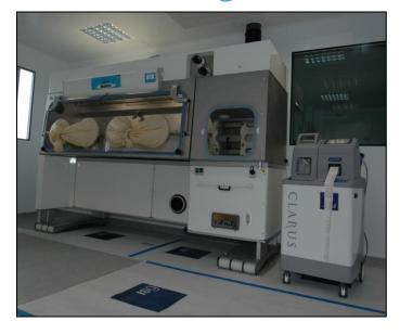
Amercare Gassing isolators are designed to provide a GMP environment for a wide range of applications including.
